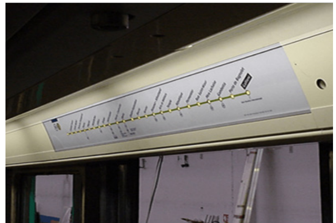
Visual panel in Paris metro displaying train position provided by MOL81/OMR equipment
