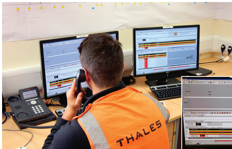
A temporary control centre at Old Dalby (left) is linked to a signal equipment room housing the System Management Centre and the Vehicle Control Centre which provides the core interlocking functions (right).
